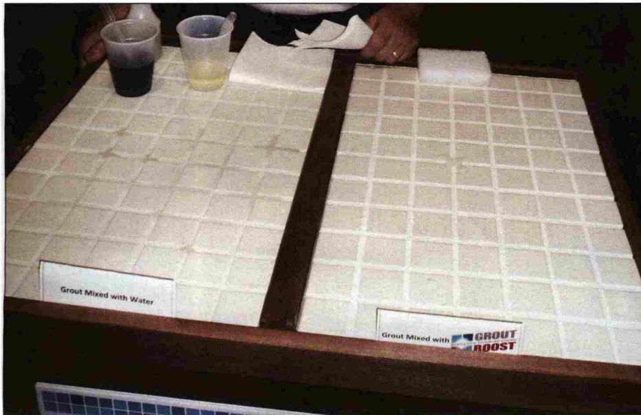
Grout Boost's additive makes cement-based grouts resistant to stains without sealing.
