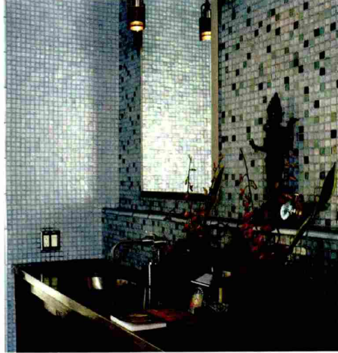
Oceanside Glasstile is made from silica sand, an abundant natural resource, and up to 86 percent recycled material, including more than two million pounds of glass from curbside recycling programs.
